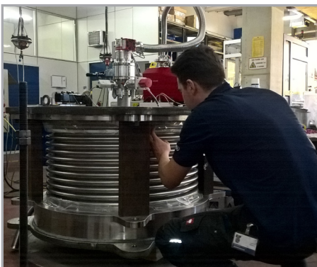
Factory acceptance testing of bellows. Image: ITER Organization
